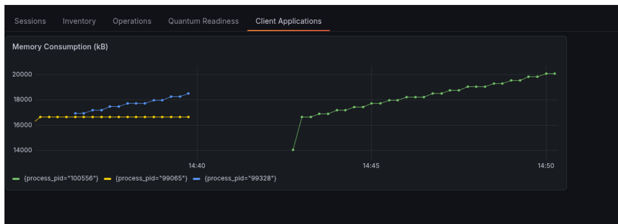
Figure 7 : Dashboard - Client Applications (memory leak detection)
